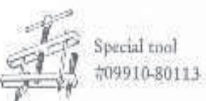
Set the crankcase separating tool on the left crankcase as shown in the figure. Separate the crankcase into right and left halves by screwing the handle of the special tool in. At the same time, push in the engine oil pipe at the right side of the case so as not to damage it.
